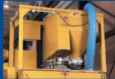
1 Load cells on each corner of weigh batcher provide accurate weighing for precise batches every time
