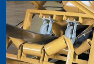
3 Adjustable hold-down wheels make for a smooth bend in belt so that one conveyor can be used to reduce costs and maintenance.
