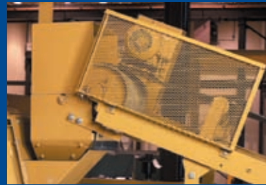
2 Conveyor guard protects operator from moving parts. Adjustable belt cleaner on conveyor head pulley keeps belt and plant clean.
