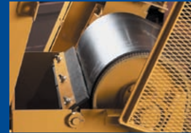
2 Conveyor guard protects operator from moving parts. Adjustable belt cleaner on conveyor head pulley keeps belt and plant clean.
