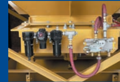
4 Aggregate gate is controlled with an electric solenoid valve and air cylinder to maximize speed and accuracy. Vibrator location allows smooth flow of aggregates regardless of moisture content; adjustable gate stop helps fine tune material flow.
